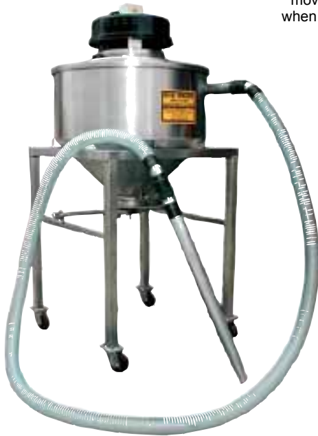
This stainless steel vacuum unit was designed to speed up the daily cleaning routine in a chicken processing plant.
